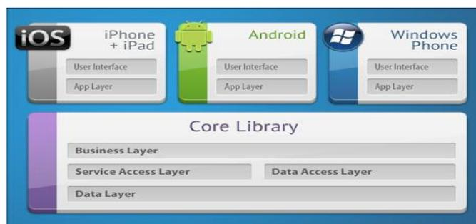
**Fig.8. Technical architecture of Xamarin platform**
