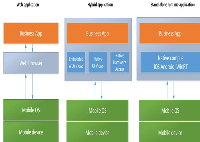
**Fig.1. The technical architecture technologies of cross-platform mobile applications development**
