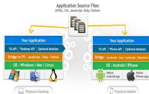
Fig.6. Technical architecture of Appcelerator Titanium
