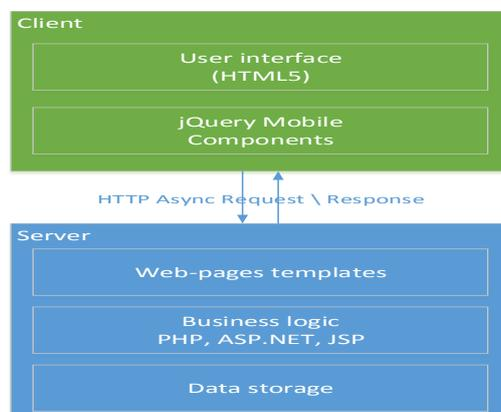
Fig.2. The architecture of mobile web applications jQuery Mobile
