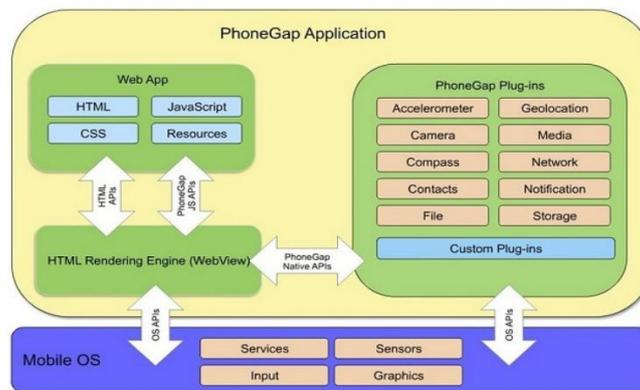
**Fig.5. Technical architecture of a hybrid approach to development mobile applications**
